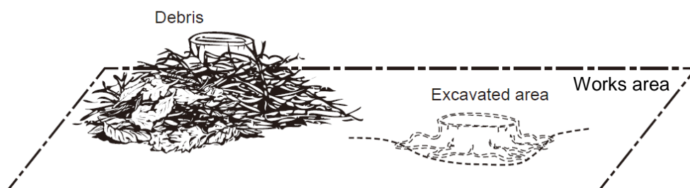
Removing and handling the stump, roots and associated soil
