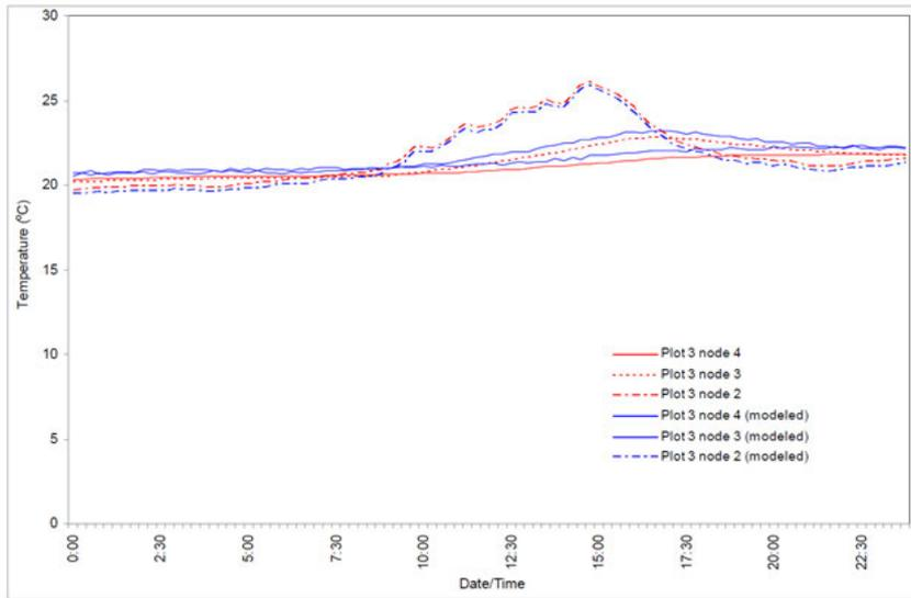
Fig. 9. Comparison of daily modeled and measured temperatures at nodes 2-4 of Plot 3 on a sunny day after a rainy day (28 March 2008).
