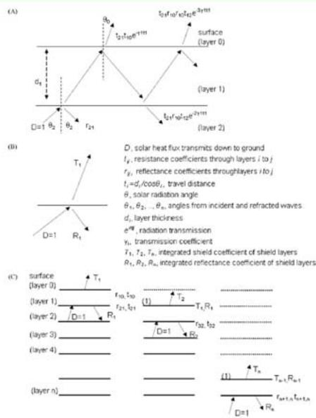
Fig. 1. The parameters involved in the radiation shield effectiveness of green roof vegetation. A: process of single-layer radiation transmission; B: computational model of single-layer shielding; C: computational model of multi-layer shielding.
