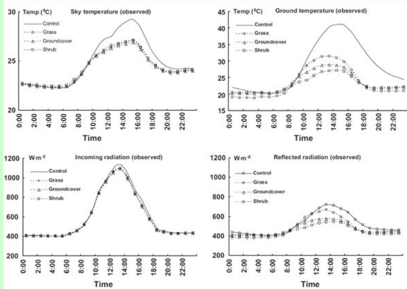
Fig. 3. Observed heat flux daily cycles of the experimental green roof plots in 2008.
