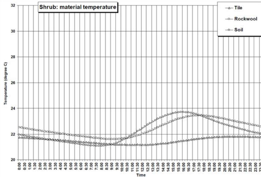
Fig. 12. Material temperature in the soil, rockwool and tile layers at the shrub green roof sites.
