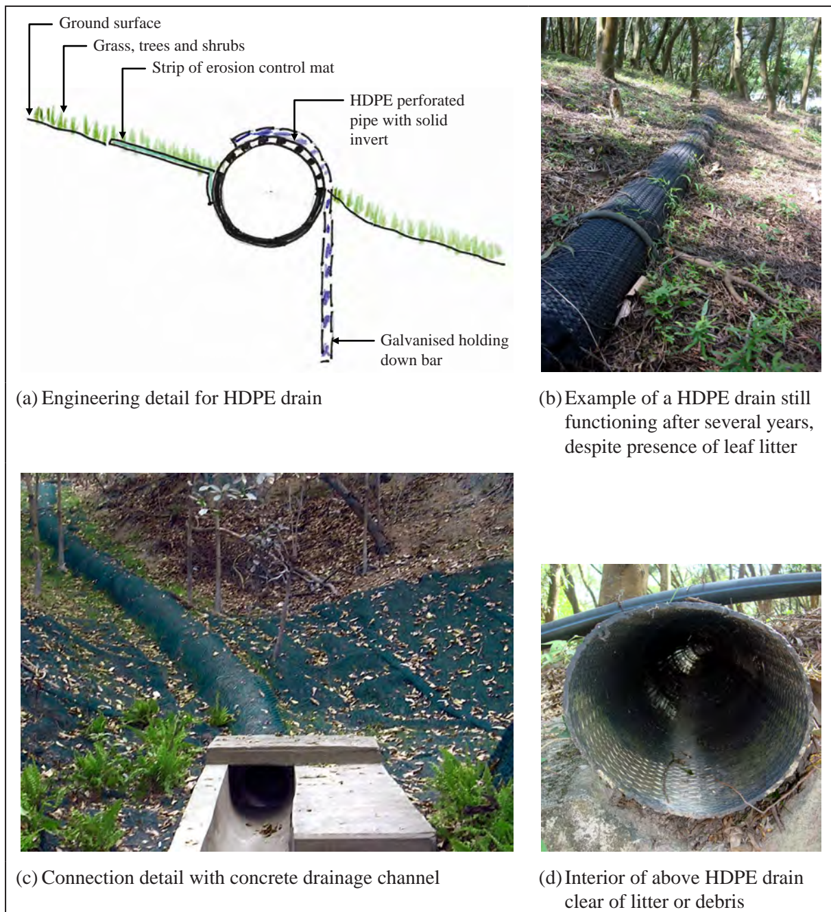
Figure 6.2 Alternative HDPE Surface Drain Pipe
