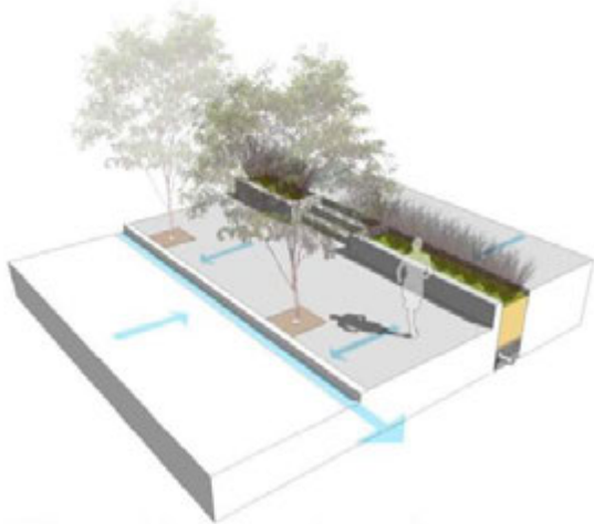
Plaza bioretention planter
