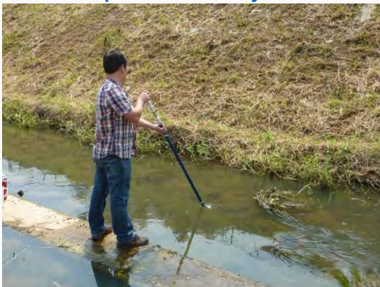
Flow metering at Ma Wat River
