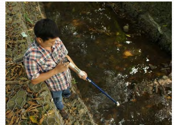
Flow metering at Ping Yuen River
